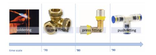
The modern time in pipe jointing technology began in the 70s and 80s with the increasing use of plastic pipes in hot water applications.
